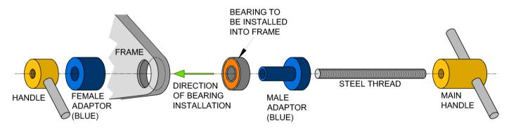
Wind on the main handle until all the parts come together, the male adaptor should be pressing on the outer race of the bearing you are inserting. Make a final check that everything is aligned properly.
